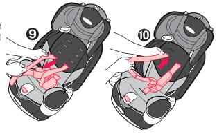
8. Use plastic strap guides as a guide to feed the harness up over the red rollers. Make sure to feed straps *OVER* red rollers and plastic strap guides 1.
